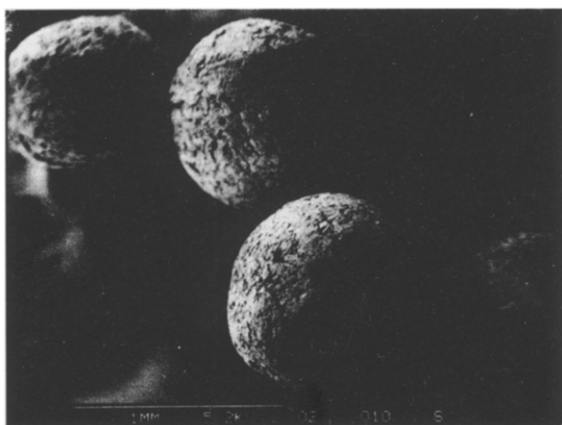
Fig. 2. Scanning electron micrograph of the shellac microcapsules. (Cambridge Stereoscan S 250, Mark III, scan time 60 s).
